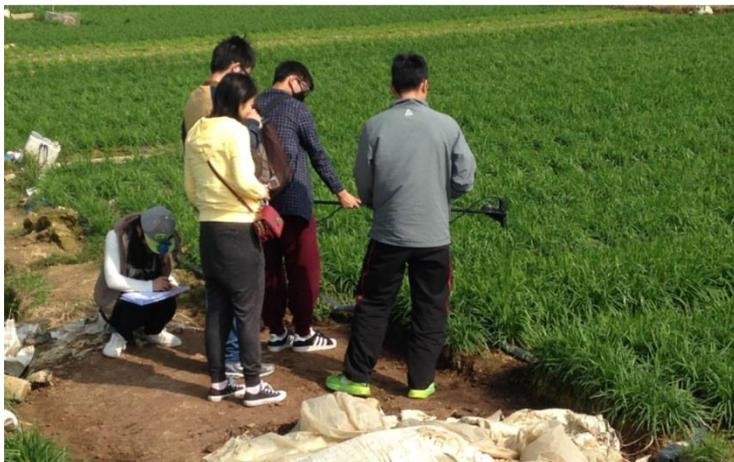
Figure 2. Collection of spectral reflectance on farmland using an ASD spectrometer
